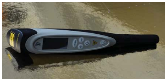
Figure 1. The handpiece of the DDPen.
