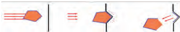
Figure 6. The principle of CoJet treatment: the silica coated alumina particles create micro roughness of the surface due to the kinetic energy and leave silica embedded inside the surface, so it can react chemically with a primer (Silane) [21].
