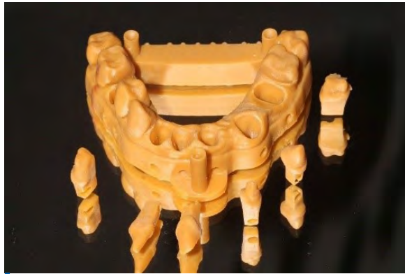
Figure 7. Polymer model made by 3D printing from digital data.
