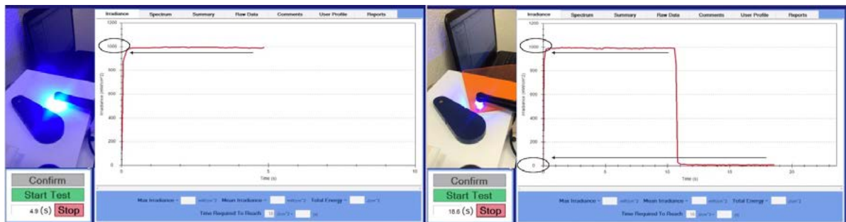
Figure 5. Effect of blocking blue-light irradiance from a multi-wave light curing unit during light exposure.
