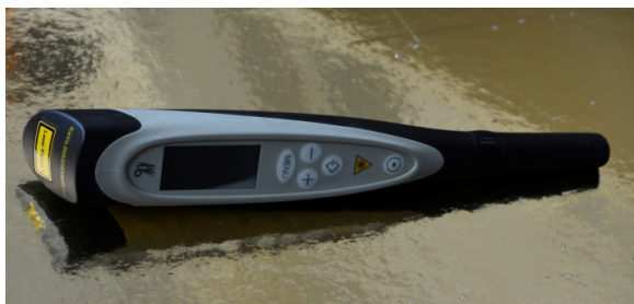
Figure 1. The handpiece of the DDPen.
