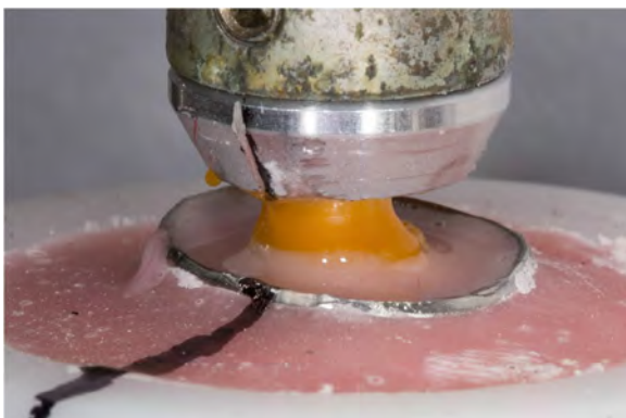
(c) Lowering the mouting jig arm to position specimen teeth into cold-curing acrylic resin.
