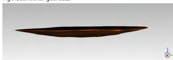
(d) Lateral view: the space within the facet was filled in creating a flat surface above in level with the non-worn periphery; it resembled the surface before starting wear simulation.
