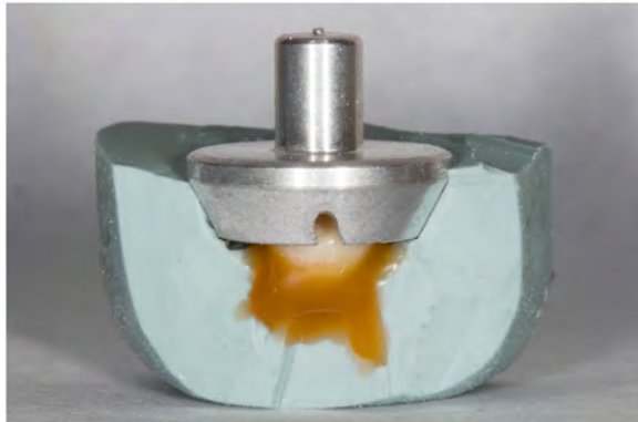
Figure 1. Use of a polyvinyl siloxane putty jig to achieve consistent relationship between the antagonist teeth to their holders. Note the mechanical retention on the antagonist holder to obtain a rotation lock.
