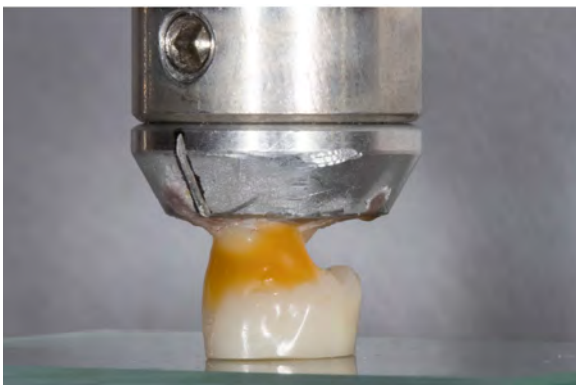
(b) A specimen tooth was stabilized onto its antagonist tooth using a dental stick wax.
