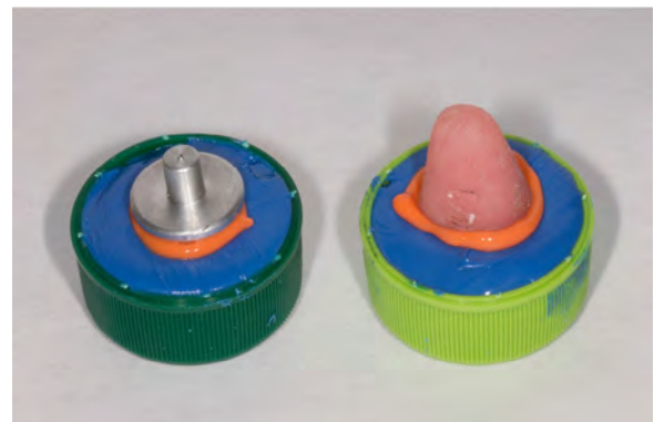
(a) Impression making of an antagonist tooth (left) and a specimen tooth (right).
