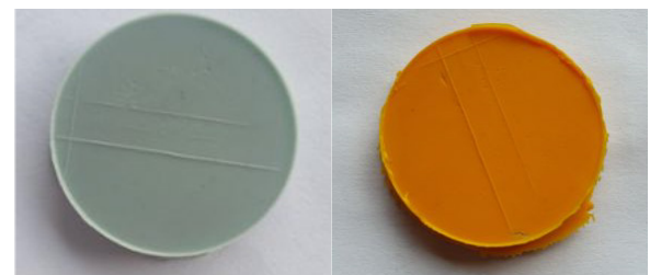
Figure 1a. Siloxane polyvinyl samples: a. condensation with medium fluidity.
