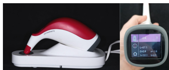
Figure 6. The VITA Easyshade V spectrophotometer measures L^*a^*b^* values.
