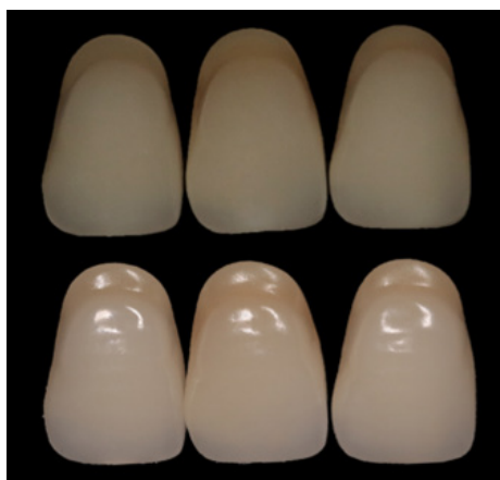
Figure 11. D2 shade tabs. Reference shade tab on the left side. Discolored shade tabs on the middle and on the right side. For the upper pictures a cross polarization filter was used to remove glare.
