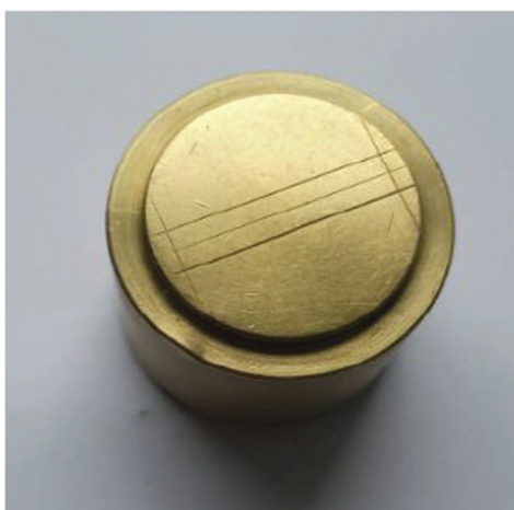
Fig. 3. Magnified image of the mold from which the samples were obtained.
